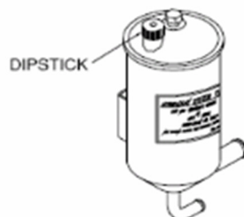
HYDRAULIC FLUID RESERVOIR
