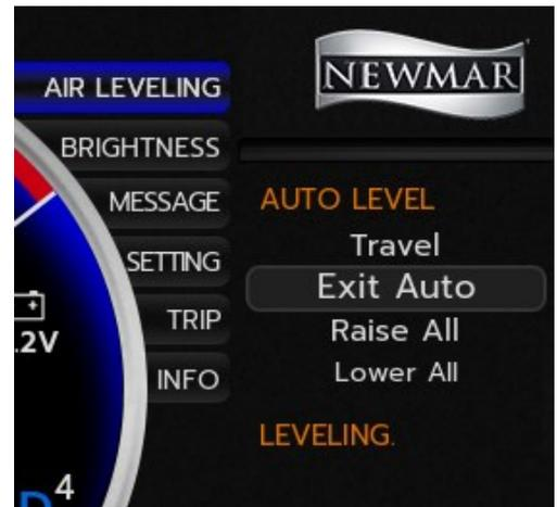
Once leveling has been completed, additional leveling cycles can be performed if the system is in auto mode or auto low power mode.
