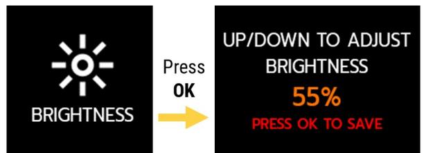
Use the **Up** and **Down** buttons to adjust the brightness and then press **OK** to save for that mode and return to the previous menu. If the marker lights are off, the brightness will be set for daytime driving. If the marker lights are on, the brightness will be set for nighttime driving.
