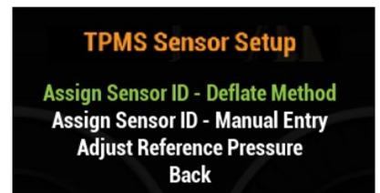
2. Exit the coach and deflate the tire by at least 5 psi. This action triggers the TPMS to select the tire for ID assignment.
