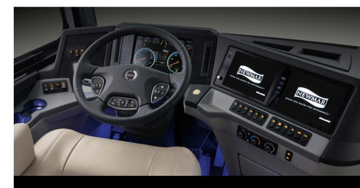
Features included in the Tri-Pod Steering wheel include windshield wiper controls, phone and media controls, steering assist functions, graphic instrument cluster navigation, cruise control, and more.
