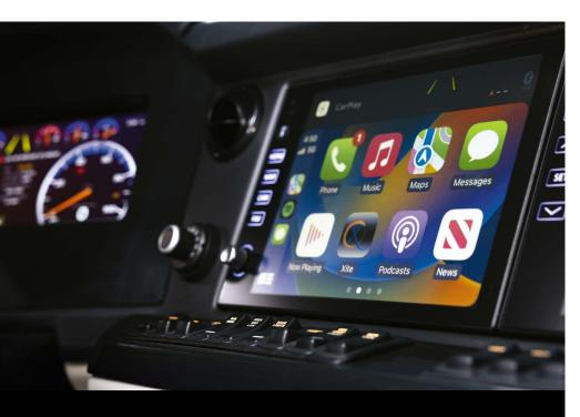
The digital dash integrates with the Tri-Pod Steering Wheel and is engineered to receive direct, clear notifications from the Spartan® RV Chassis Advanced Protection System™, a suite of comprehensive safety technology. Advanced Protection System features include: Collision Mitigation, Adaptive Cruise Control, Electronic Stability Control, Automatic Traction Control, Tire Pressure Monitoring System, and Lane Departure Warning.
