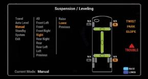
Electronic ride height and air leveling system integrated into the digital dash.
