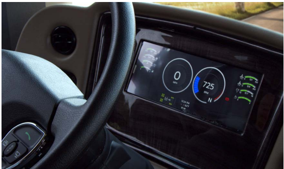
Spartan's Connected Coach™ digital dash system combines an intuitive interface with custom graphics and information. Entegra motorhomes riding on a Spartan chassis also have the convenience of keyless entry and push-button start technology.*
