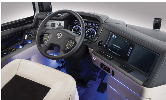
Spartan's Connected Coach™ digital dash system combines an intuitive interface with custom graphics and information, plus the convenience of keyless entry and push-button start technology.
